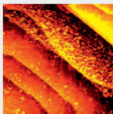
Graphene and O(2x2) on Ru(0001) imaged at 10 mbar in Nitrogen atmosphere: T=500 K, I=0.7 V, U=0.7 V
